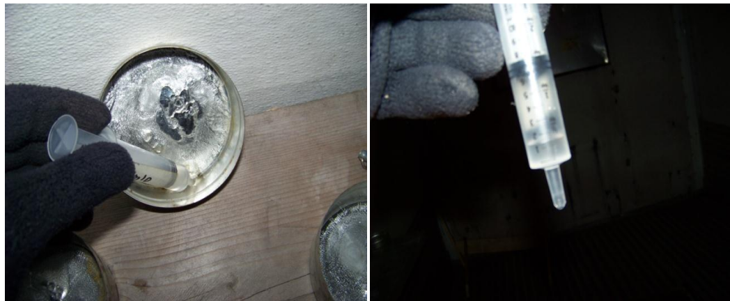
Figure 3.16: Refreeze Test Liquid Measurement
